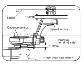
The maximum distance between the speed crank and the magnet is 5mm, same as between the cadence sensor and the magnet.
